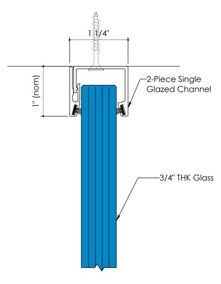
Solare <sup>™</sup> Acoustic Single Glazed Partition System Standard Track Head
